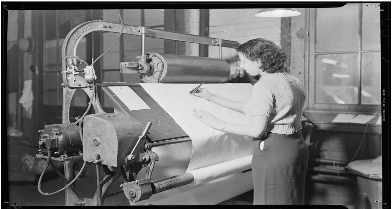
Fig. Fabric inspection
